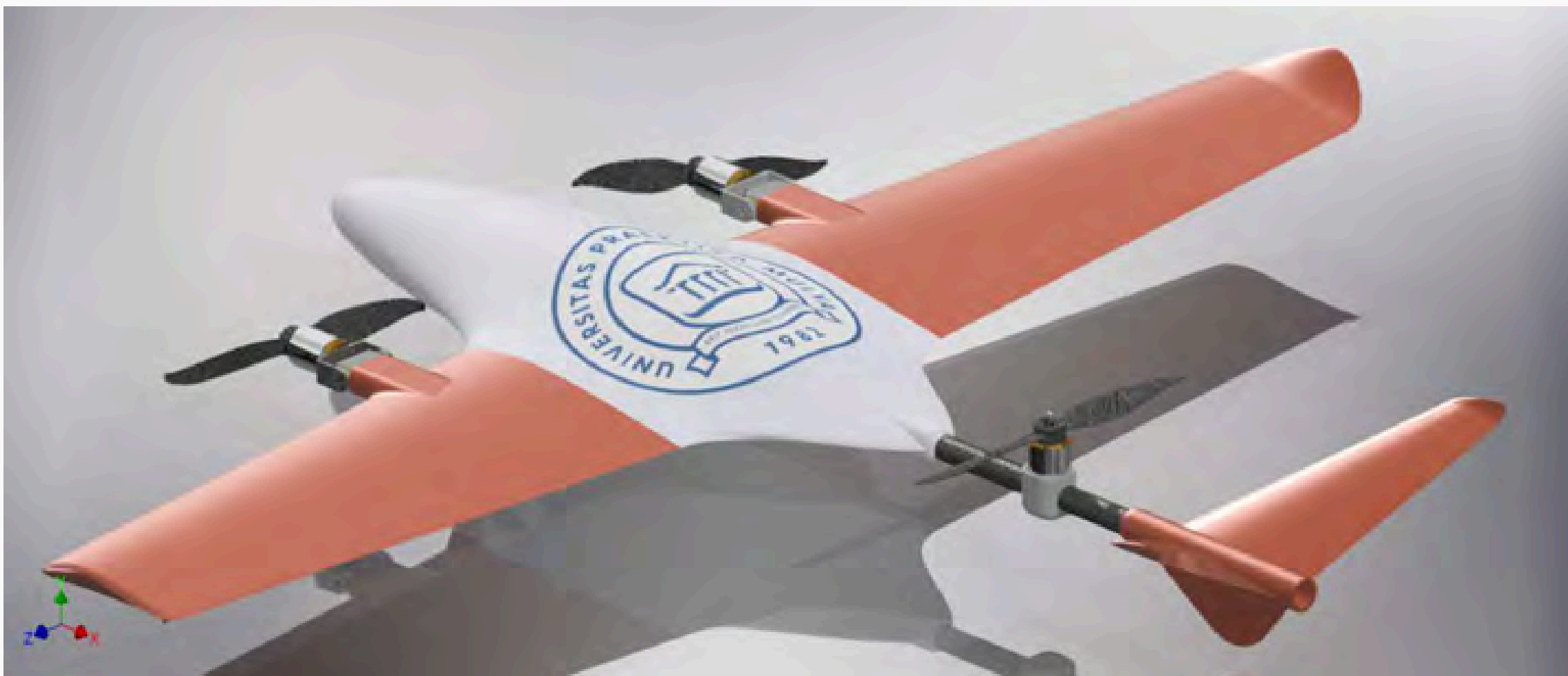
Gambar 2. Design of Fixed-Wing Hybrid Tricopter UAV
